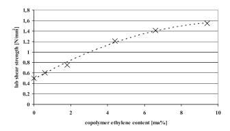
Lab shear strength of poly(butene-1) (ethylene content = 0 ma%) and poly(ethylene-co-butene-1) solution polymers on untreated poly(propylene).
