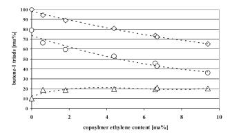
**Figure 4.** Absolute content of butene-1 triads ( $\diamondsuit$ ), isotactic butene-1 triads ( $\bigcirc$ ) and atactic butene-1 triads ( $\triangle$ ) of poly(butene-1) (ethylene content = 0 ma%) and poly(ethylene-co-butene-1) solution polymers. Reaction conditions: T = 115 °C; solvent: n-butane; catalyst: 0,1 g TiCl<sub>3</sub>\*AlCl<sub>3</sub> per 1.000 g monomer(s), cocatalyst: 5.50 g triisobutylaluminia per 1 g catalyst.
