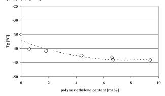
**Figure 3.**♦ DSC glass transition temperatures (second heating) of poly(butene-1) (ethylene content = 0 ma%) and poly(ethylene-co-butene-1) solution polymers. Reaction conditions: T = 115°C; solvent: n-butane; catalyst: 0,1 g TiCl<sub>3</sub>\*AlCl<sub>3</sub> per 1.000 g monomer(s), cocatalyst: 5.50 g triisobutylaluminia per 1 g catalyst.
