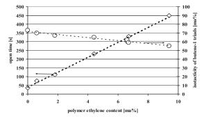
**Figure 5.** Open time ( $\diamondsuit$ ) and rel. butene-1 triad isotacticity ( $\bigcirc$ ) of poly(butene-1) (ethylene content = 0 ma%) and poly(ethylene-co-butene-1) solution polymers. Reaction conditions: T = 115 °C; solvent: n-butane; catalyst: 0,1 g TiCl<sub>3</sub>\*AlCl<sub>3</sub> per 1.000 g monomer(s), cocatalyst: 5.50 g triisobutylaluminia per 1 g catalyst.
